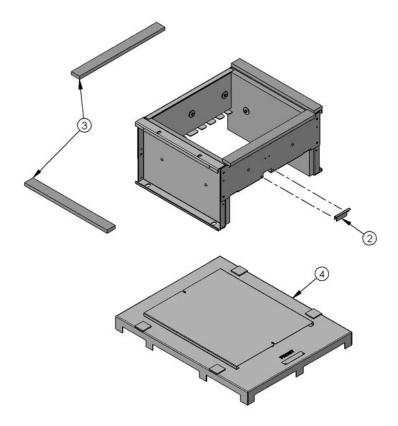
Figure 11.1: Base/Combustible Floor Pan
